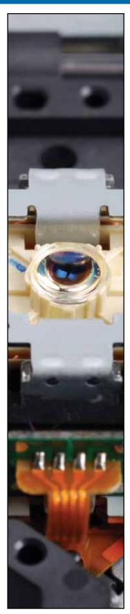
Detectors consist of a photodiode, amplifier, voltage regulator, Schmitt trigger, and output stage with a 10 kOhm pull-up resistor, open collector, or totem-pole output. IR LED sensors facing Optoschmitt detector in plastic molded housing – switching occurs when opaque object passes between emitter and detector. Digital output used for presence/ motion sensing and encoding.
